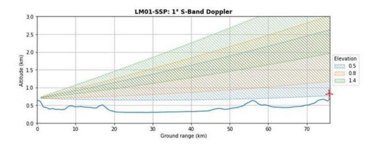
Caption: Preliminary impact assessment on S-Band weather radar at Namoi weather station. Source: Bureau of Meteorology (2021)
