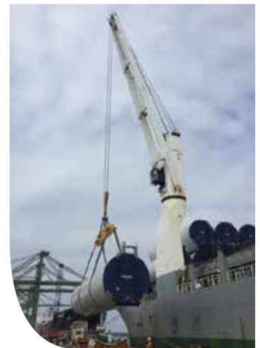
Turbine tower section being loaded.
