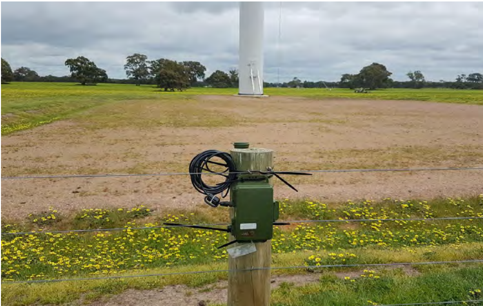
Figure 2 SM2 detector mounted on a fence near Turbine 13
