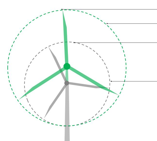
Varied Project: Tip height up to 220 metres — Varied Project: Indicative rotor diameter up to 180 metres Approved Project: Tip height up to 165 metres
